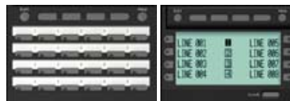
Interchangeable function modules — 24/32 button and dual screen LCD
