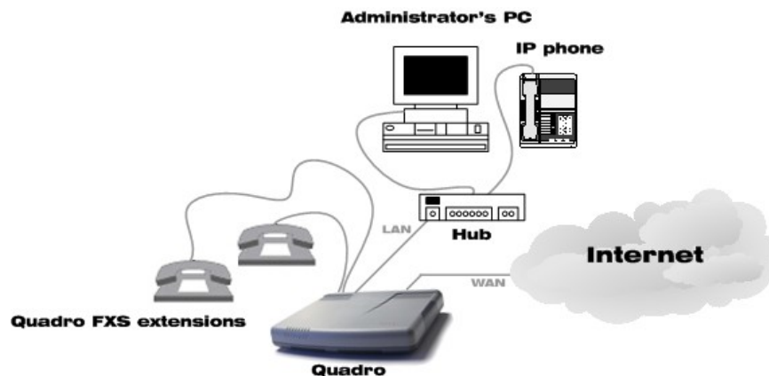
Figure 1 IP phone connected to the Quadro LAN
