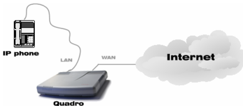
Figure 5 IP phone obtains basic network parameters from the Quadro DHCP server
